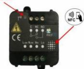
To use the NFC interface, the device must be powered through terminals L LINE and N LINE. The power status is visible on the red/green led. Alwaysvalidate your settings by reading the NFC data after the sensor has restarted.
